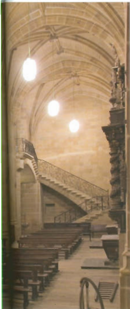
Viewing the altar from the pews, the observer is not affected by glare from the luminaires mounted on the columns. This is not the case for the priest, choir and servers.
